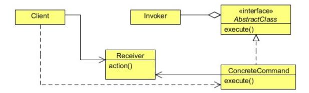
Figure 20.1: - Command pattern Class diagram
